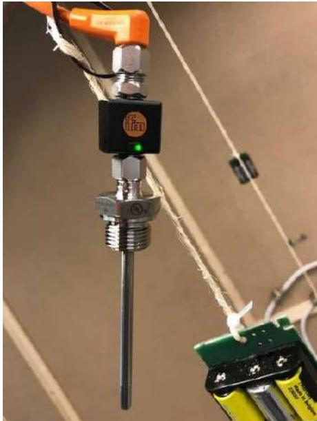
← In the centre of the test-room a temperature sensor was installed, acting as the room thermostat
