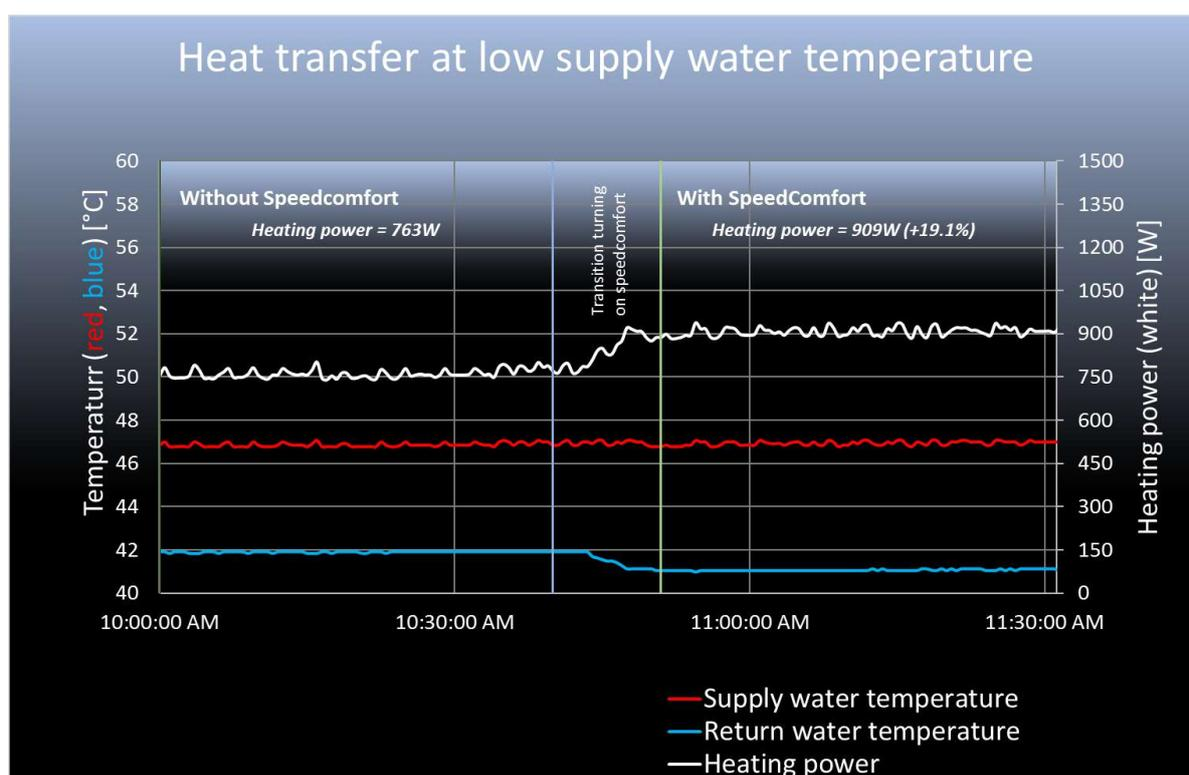
The increase in power transfer induced by SpeedComfort is a result of increased heat transfer from heating panel to air. This heat transfer is given by the following equation:
