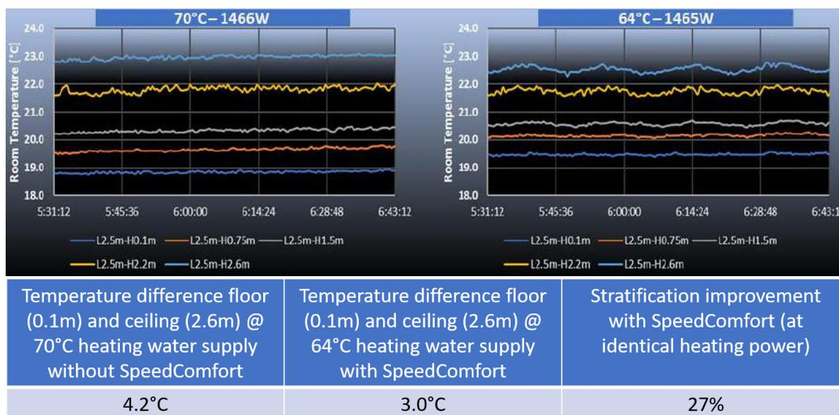
The graphs show that a **stratification difference of 1.2°C** (4.2 -/- 3.0) is created by assisted convection: temperatures at ceiling level come down, whereas those at the bottom of the room (‘feet level’) reach higher levels. This indicates a better warmth distribution on those locations where people will notice it (0.1m < 2.0m). Apart from the actual increase in temperature in the living zone, it will also add to the personal factors/drivers of thermal comfort (‘warmer feet’).
