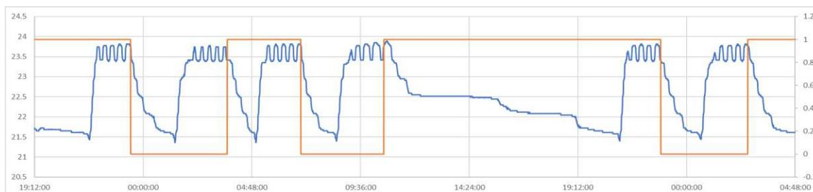
The above test results show that the improved warm-up time is 16% at 1.3°C and 41% at 2°C. Energy consumption is slightly lower (-3%) at 1.3°C but significant at 2°C (-24%).
