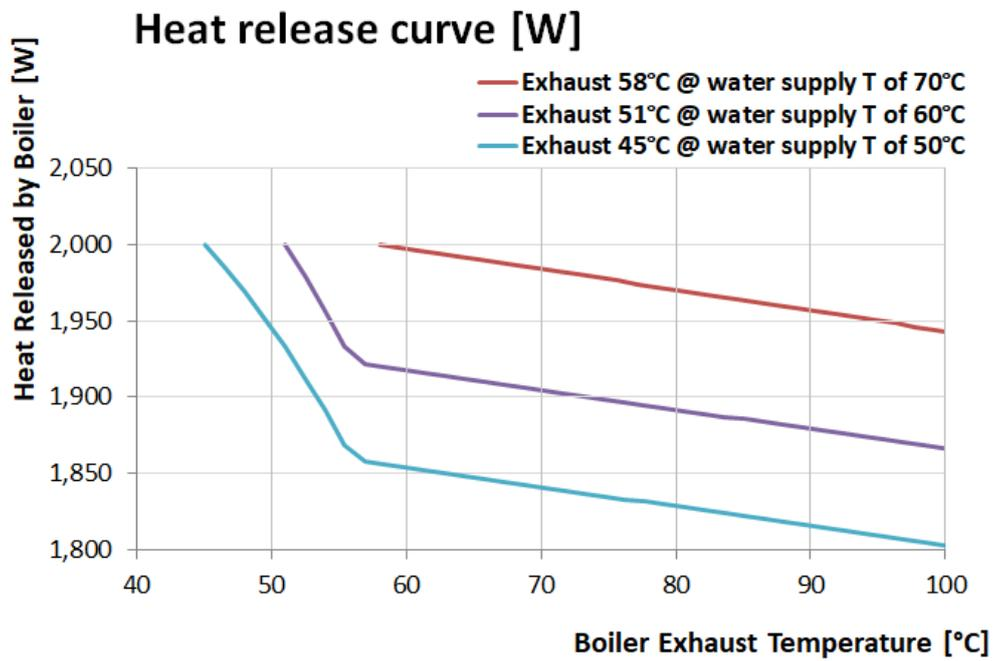
By proper utilization of the SpeedComfort units, gas consumption for heating can be reduced by around 2% by turning the supply water temperature down, without taking any other saving measures.
